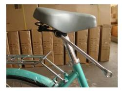
Tighten the bolts on opposite sides of the seat post connector with a 14mm or adjustable wrench. Alternate sides after each rotation to tighten evenly: tighten one side a full rotation, then the opposite side a full rotation, and vice-versa until each bolt is completely tight and there is no movement in the saddle angle.
