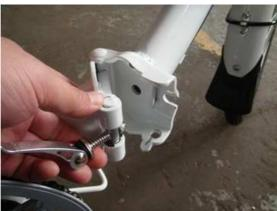
When unfolding, swing your frame together. Make sure the quick release bolt snaps into the frame folding box.
