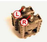
Your bike includes a set of pedals. The pedals are marked on the end of the pedal axle: "R" for "Right" and "L" for "Left." When seated on the bike, your right foot would correspond to the right pedal and your left foot would correspond to the left pedal.
