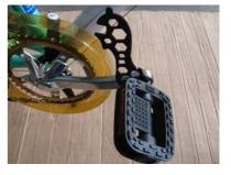
Please note you need to screw the right pedal clockwise into the crank eye, and screw the left pedal anti-clockwise into the crank eye. If it does not turn easily do not force it and double check that you have choosen the correct pedal doing in a correct way. Forcing the wrong pedal going in will damage the thread on your pedal and crank arm.
