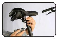
11: Install the saddle and lock the screws with a tool 12: L-Left Pedal. Tighten left pedal anticlockwise.
