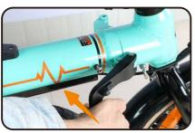
6: Twist the handlebar to the best angle
